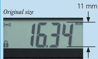
The high-contrast display with 11 mm high digits enables accurate, fatigue-free reading of the measurement results.
